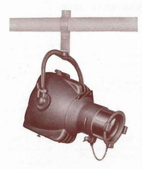
This is a small, compact lantern with a multitude of applications in stage lighting, picture lighting, shop window display, exhibition work and the like. It gives a clear-cut beam of any required shape and free of stray or ghost light. The lantern has been completely tooled for mass production with die-castings and consequently represents exceptional value for the price.
